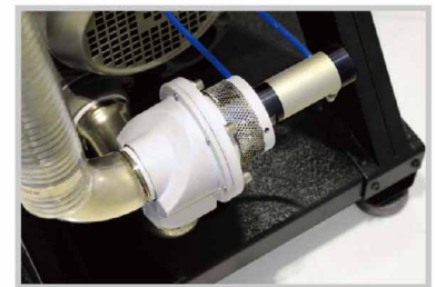
Vacuum breaking valve
