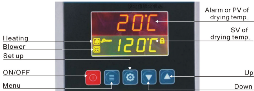
Picture 4-1: Control Panel
